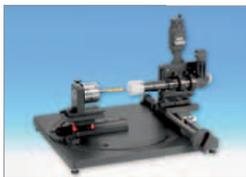
The V-block is replaced by a mounting device for a Röh chuck (ZG dia. 80 – ID 146 195 – for up to 19.5 mm) on the motion carriage and arrested at the bottom with a knurled screw. The Röh chuck is also available with the holding device, if required.
