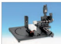
Measuring the edges of the diameter or the thread pitch with top light or diffuse bottom light presents problems. On rotationally symmetrical objects no distinct edges are obtained, or, expressed differently: The light "creeps" around the edges reducing the diameter of the specimen in the image. For such measuring tasks we use a parallel bottom light to prevent such problems. A blue LED is used, because blue has the lower deflection.
