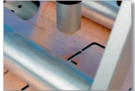
The virtually play-free, coaxial drive allows exact focussing on the focal plane. Important for optimum readings: Always focus the top and
