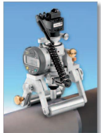
The MST stand provides a secure position on drums or flat material for depth measurement. An additional five millimetre X-adjustment at high magnification allows feed motion between the focal planes, when they can no longer be covered by the field of vision. In addition to visualisation the Metric Standard or Metric Plus measuring software allows 2D measurements, such as distances, angles, radii and areas.
