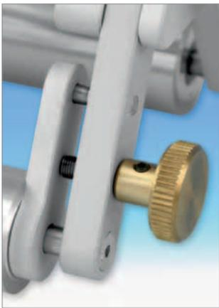
the only feature that allows exact recognition of the focal planes. The fine focusing mechanism can be pushed to the side for quick adjustment. An LED ring light is included with the set for materials such as rubber. The nine LED's are arranged at an angle of 30° to the optical centre.
