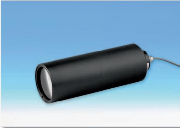
Telecentric illumination is a special form of focussed illumination with high directional characteristics. This application is accomplished almost exclusively using transmitted light. A light source (usually LED) of known, small illumination aperture is positioned in the focal plane of the light's optical system. The result is parallel chief rays. Telecentric lighting is not parallel lighting (defined aperture). This makes it considerably less sensitive to vibration or maladjustment.
