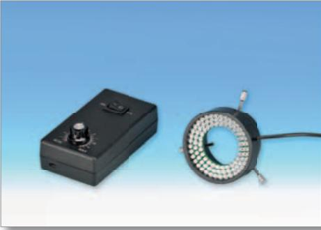
In any applications LED ring lights are perfectly sufficient for top lighting. The CV-LED-R with its 98 white LED's, arranged at an angle of 15° in three rows, offer perfect illumination quality. The outer diameter is 67 mm and the inner opening 35 mm (see drawing). The set included a power supply with infinite dimming feature.
