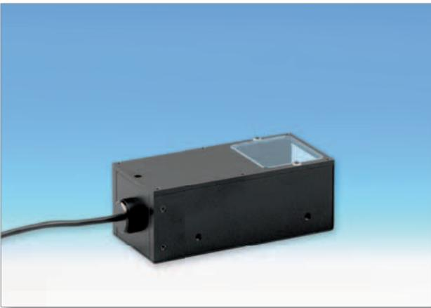
It is no longer possible to use normal diffuse light to measure the diameter of rotationally symmetrical parts or the pitch on threads and taps, because the lights cannot "bend" around the edges, so that the diameter is indicated as less than it is in reality. Parallel bottom light can be used for such applications, because it guarantees that the light comes straight from below making precise measurement possible. The light from the blue LED (blue = least deflection) is guided
